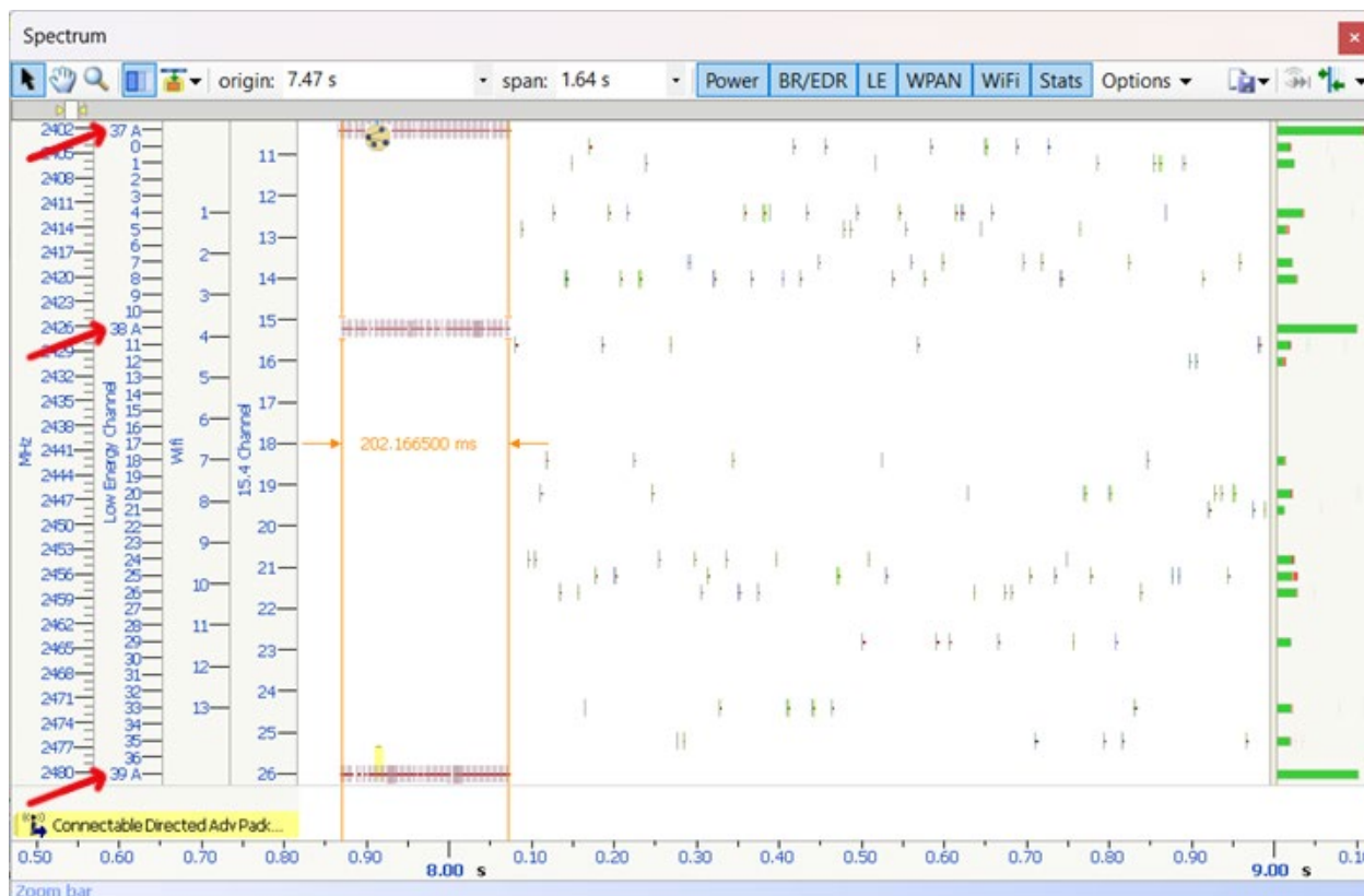
Figure 1 The Spectrum View of the Ellisys Bluetooth Analysis Software showing ADV packets in the three primary advertising channels.
